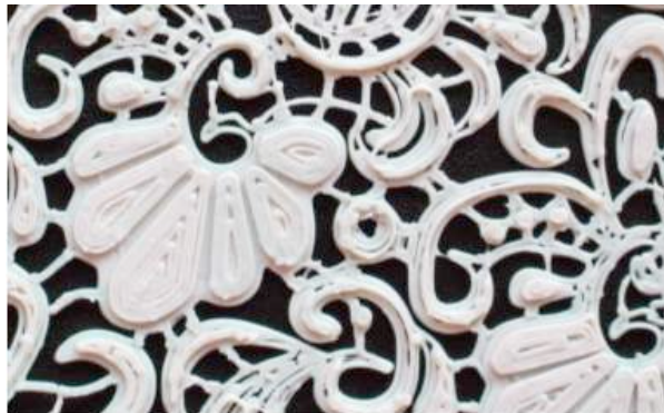
Figura 8: Textura impresa en 3D. Fuente: Ehrmann, A y Finsterbusch, F. (2014). 3D printing of textile-based structures by fused deposition modelling (FDM) with different polymer materials. Disponible en: http://iopscience.iop.org/article/10.1088/1757-899X/62/1/012018/pdf
